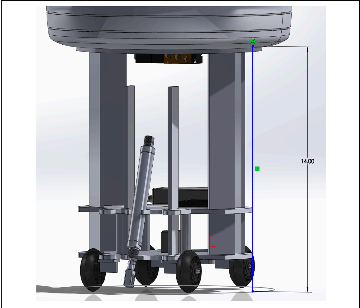
Figure 8: Dimensioned view showing height between top of tire plate and bottom is 14"
